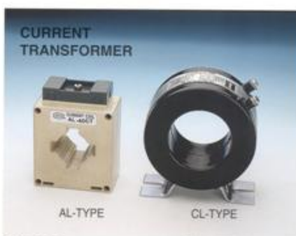
AL TYPE Model: AL-TYPE Range: 10-3000 / 5A Rated burden: 3VA & 5VA Acc class: 1.0 Insul class: 0.6 kv
